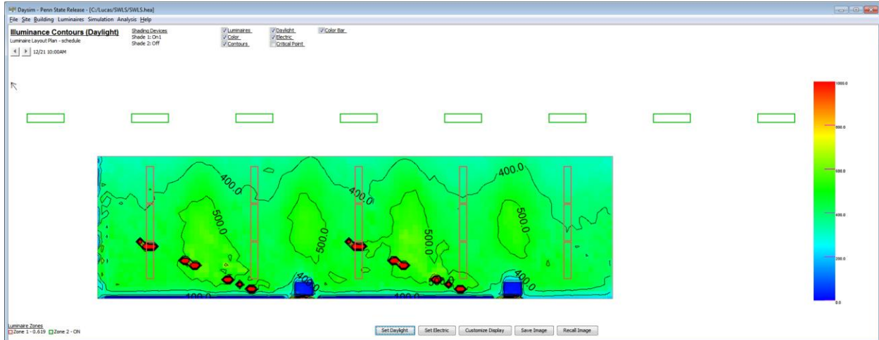
Illumination Contours for the Southwest Facing Life Science Façade (12/21 – 10:00AM).
